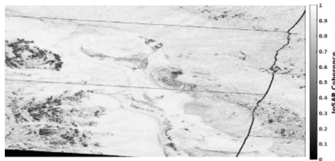
Figure 3: InSAR coherence map generated directly from Figure 1 and Figure 2
